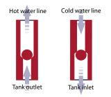
If **anti-convection valves** or **heat traps** for both the cold-water inlet and the hot water outlet are not included with your new water heater, make sure the installer adds them. **Electric offers low initial cost**
