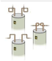
Heat traps fabricated from copper plumbing pipe can help prevent heat loss from a storage-type water heater.
