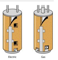
Wrapping an **insulation blanket** around the tank of your existing gas or electric water heater can save you money on water-heating bills. The insulation blanket will reduce standby heat loss—heat lost through the wall of the tank—by 25% to 45%, and you'll likely recover the cost of the blanket through reduced water-heating bills within a year.
